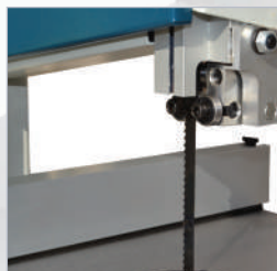
Guías de sierra Saw guides Guides de lames
